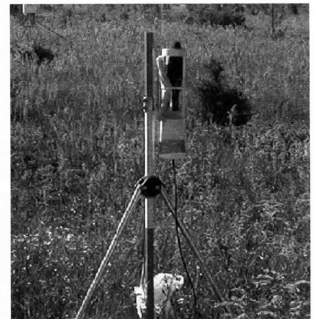
Figure 4. Microphones were surveyed to a constant height above ground and protected with acoustic foam to reduce wind noise.
